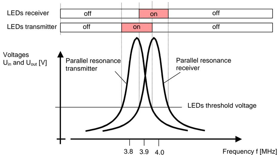
Figure 8: Dependency of the LEDs glowing on the frequency of the HF source.
