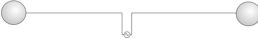
Figure 4: HERTZ dipole
