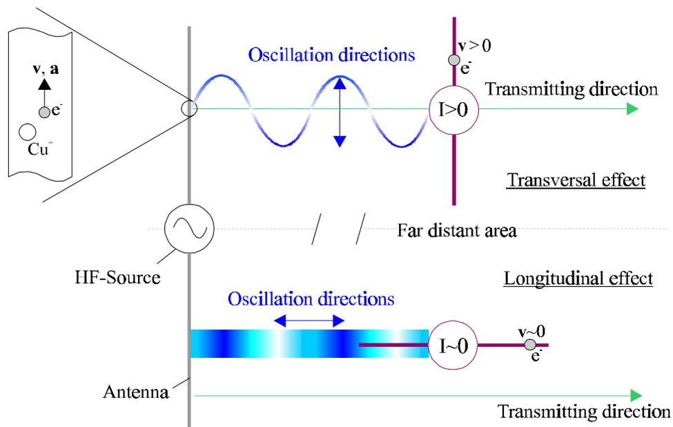
Figure 2: Difference of transversal and longitudinal effects of a HERTZ transmitting antenna to a far distant charge  $q^+$ .
