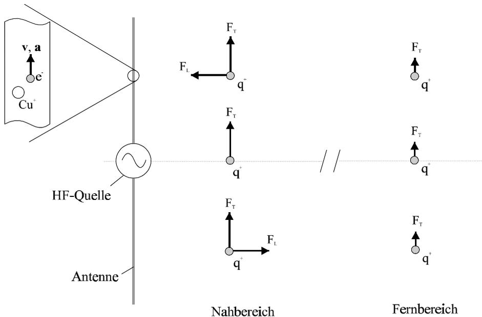
Figure 1: Force of a transmitting antenna on a distant test charge  $q^+$ .
